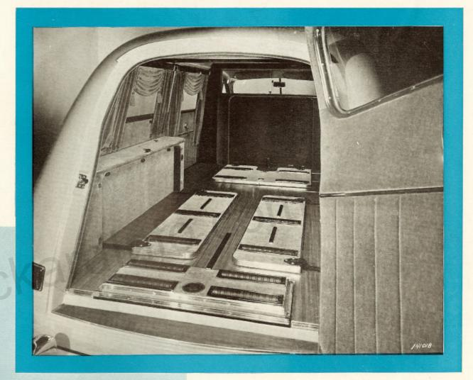
This illustration, taken thru open rear door, shows the roomy body — full size in each dimension —and the simple but quick acting method for lowering the casket table panels when converting for hearse use.
